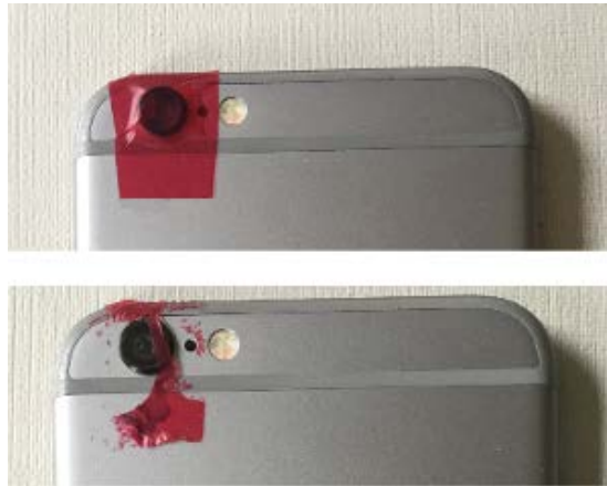
Figure 3: Sealed smartphone camera (intact and broken)
